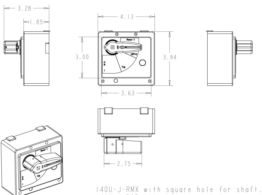
140U-J-RMX with square hole for shaft. 140U-J-RCB without square hole. Otherwise dimensionally the same.
